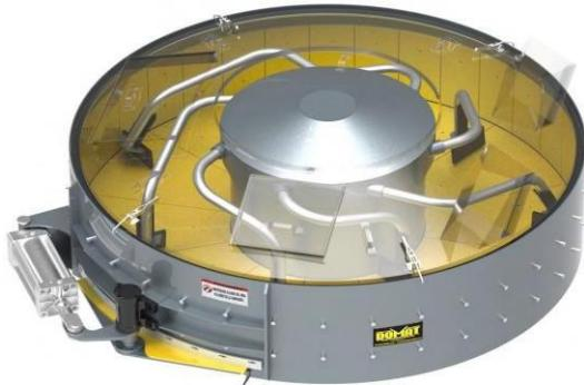
DOMAT turbo vertical axis mixer with capacity of up to 0,65 Yd<sup>3</sup> per batch. High efficiency reduction system brand SUMITOMO (Japan) or OMCI (Italy) by vertical axis inferential coupling of the gearmotor with a power of 14,9 Kw. Access gates for washing and/or inspection. Arms made of rigid, high-resistance steel axles, cushioned to relieve overload, reinforced with anti-wear guards. Sheet floor and wall coverings, mixing paddles and gasket in the gate that are easy to replace.
