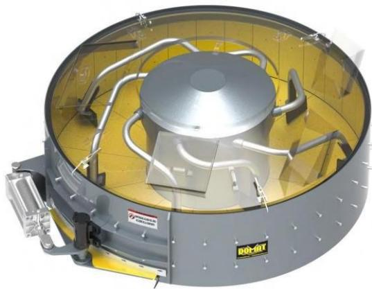
DOMAT turbo vertical axis mixer with capacity of up to 1.96 Yd<sup>3</sup> per batch. High efficiency reduction system brand SUMITOMO (Japan) or OMCI (Italy) by vertical axis inferential coupling of the gearmotor with a power of 55.9 Kw. Access gates for washing and/or inspection. Arms made of rigid, high-resistance steel axles, cushioned to relieve overload, reinforced with anti-wear guards. Sheet floor and wall coverings, mixing paddles and gasket in the gate that are easy to replace.
