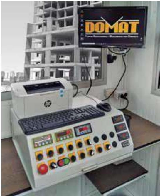
D-200 developed with an industrial computer on a Windows environment and a Siemens S7-1200 automation interface, responsible for carrying out the dosing and process control processes, meeting the necessary quality standards and effectively carried out:
