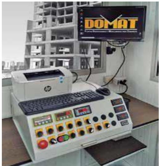
D-200 developed with an industrial computer on a Windows environment and a Siemens S7-1200 automation interface, responsible for carrying out the dosing and process control processes, meeting the necessary quality standards and effectively carried out:
