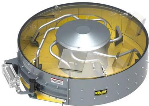
DOMAT turbo vertical axis mixer with capacity of up to 0,65 Yd<sup>3</sup> per batch. High efficiency reduction system brand SUMITOMO (Japan) or OMCI (Italy) by vertical axis inferential coupling of the gearmotor with a power of 14,9 Kw. Access gates for washing and/or inspection. Arms made of rigid, high-resistance steel axles, cushioned to relieve overload, reinforced with anti-wear guards. Sheet floor and wall coverings, mixing paddles and gasket in the gate that are easy to replace.
