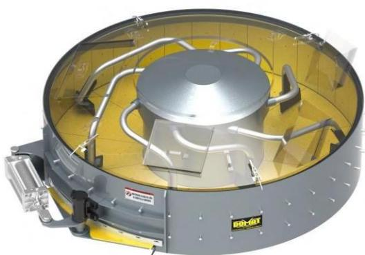
DOMAT turbo vertical axis mixer with capacity of up to 0,98 Yd<sup>3</sup> per batch. High efficiency reduction system brand SUMITOMO (Japan) or OMCI (Italy) by vertical axis inferential coupling of the gearmotor with a power of 22.4 Kw. Access gates for washing and/or inspection. Arms made of rigid, high-resistance steel axles, cushioned to relieve overload, reinforced with anti-wear guards. Sheet floor and wall coverings, mixing paddles and gasket in the gate that are easy to replace.
