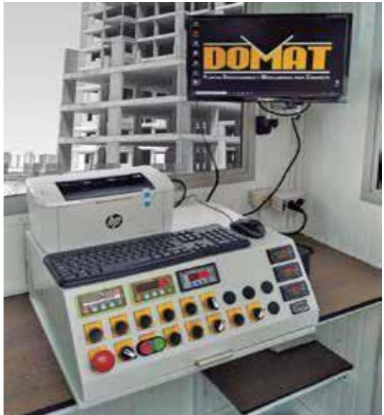
D-200 developed with an industrial computer on a Windows environment and a Siemens S7-1200 automation interface, responsible for carrying out the dosing and process control processes, meeting the necessary quality standards and effectively carried out:
