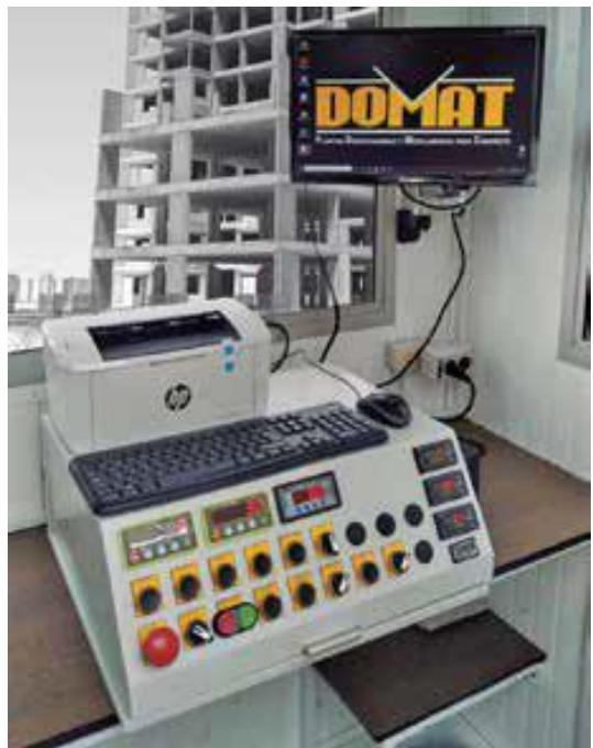
D-200 developed with an industrial computer on a Windows environment and a Siemens S7-1200 automation interface, responsible for carrying out the dosing and process control processes, meeting the necessary quality standards and effectively carried out:
