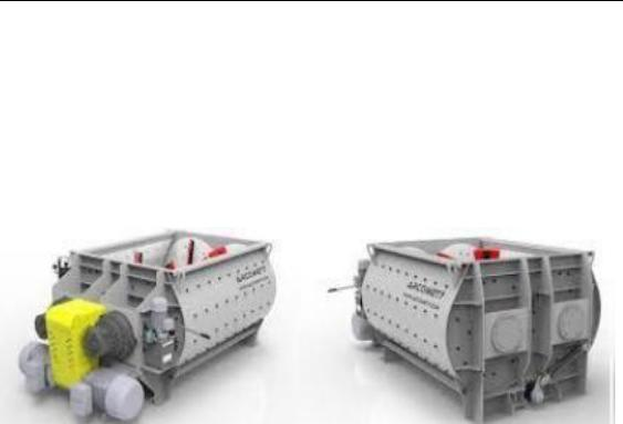
DOMAT CONTINUOUS mixers are equipped with axes that work in counter-rotation together with the mixing blades configured in angle and position that generate a double effect of mixing and translation of the material from the entry point to the discharge opening. DOMAT CONTINUOUS mixers are designed for material homogenization tasks with high efficiency and are recommended to produce mixed concrete, compacted concrete (HCR, CCR), soil-cement mixtures and fillers in the mining sector, Backfill.
