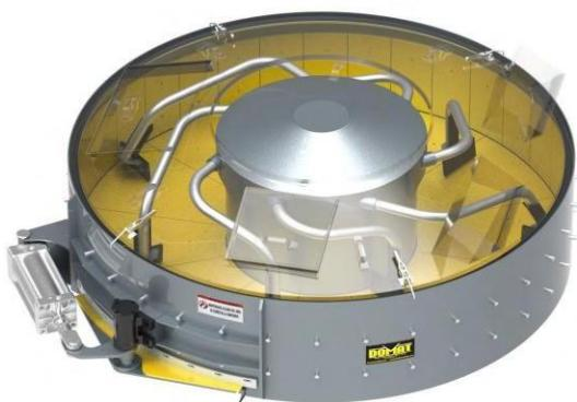
DOMAT turbo vertical axis mixer with capacity of up to 1.30 Yd<sup>3</sup> per batch. High efficiency reduction system brand SUMITOMO (Japan) or OMCI (Italy) by vertical axis inferential coupling of the gearmotor with a power of 29.8 Kw.
