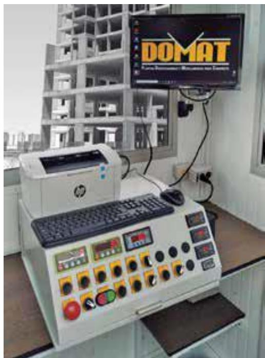
D-200 developed with an industrial computer on a Windows environment and a Siemens S7-1200 automation interface, responsible for carrying out the dosing and process control processes, meeting the necessary quality standards and effectively carried out:
