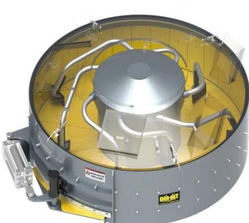
DOMAT turbo vertical axis mixer with capacity of up to 1.96 Yd<sup>3</sup> per batch. High efficiency reduction system brand SUMITOMO (Japan) or OMCI (Italy) by vertical axis inferential coupling of the gearmotor with a power of 44.7 Kw. Access gates for washing and/or inspection. Arms made of rigid, high-resistance steel axles, cushioned to relieve overload, reinforced with anti-wear guards. Sheet floor and wall coverings, mixing paddles and gasket in the gate that are easy to replace.
