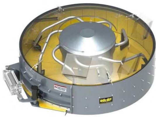
DOMAT turbo vertical axis mixer with capacity of up to 1,30 Yd<sup>3</sup> per batch. High efficiency reduction system brand SUMITOMO (Japan) or OMCI (Italy) by vertical axis inferential coupling of the gearmotor with a power of 29,8 Kw. Access gates for washing and/or inspection. Arms made of rigid, high-resistance steel axles, cushioned to relieve overload, reinforced with anti-wear guards. Sheet floor and wall coverings, mixing paddles and gasket in the gate that are easy to replace.
