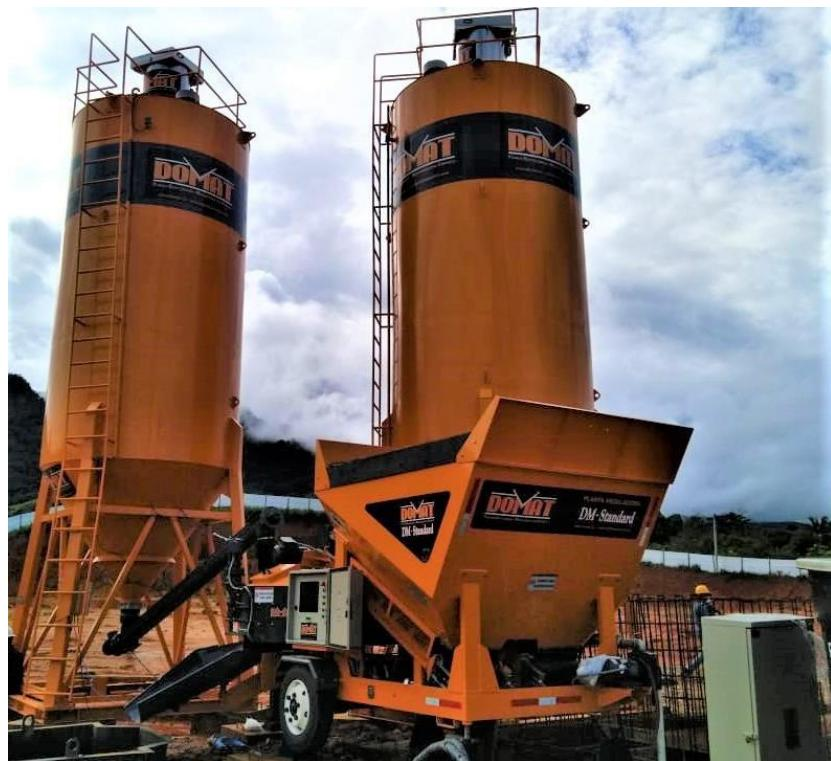
**DOMAT DM SPECIAL** concrete batching and mixing plant.
