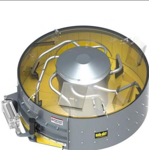
DOMAT turbo vertical axis mixer with capacity of up to 2.62 Yd<sup>3</sup> per batch. High efficiency reduction system brand SUMITOMO (Japan) or OMCI (Italy) by vertical axis inferential coupling of the gearmotor with a power of 74.57 Kw. Access gates for washing and/or inspection. Arms made of rigid, high-resistance steel axles, cushioned to relieve overload, reinforced with anti-wear guards. Sheet floor and wall coverings, mixing paddles and gasket in the gate that are easy to replace.
