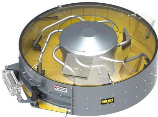
DOMAT turbo vertical axis mixer with capacity of up to 0.98 Yd<sup>3</sup> per batch. High efficiency reduction system brand SUMITOMO (Japan) or OMCI (Italy) by vertical axis inferential coupling of the gearmotor with a power of 22,4 Kw. Access gates for washing and/or inspection. Arms made of rigid, high-resistance steel axles, cushioned to relieve overload, reinforced with anti-wear guards. Sheet floor and wall coverings, mixing paddles and gasket in the gate that are easy to replace.
